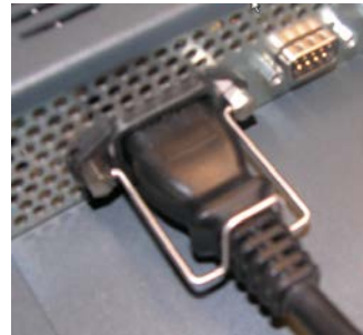
Power Cable Retention Clip Installed
