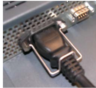
Power Cable Retention Clip Installed
