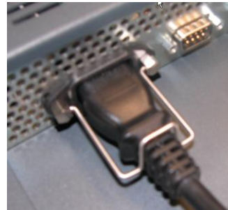
Power Cable Retention Clip Installed
