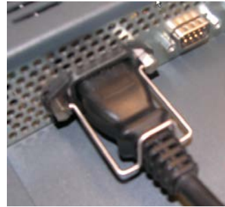
Power Cable Retention Clip Installed
